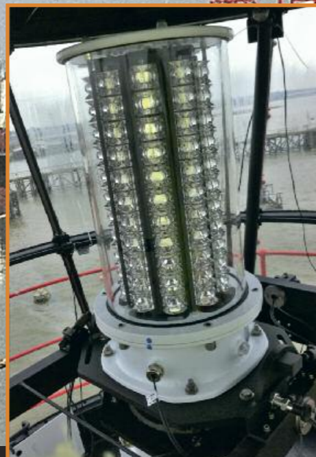
Above: In the lantern of a 20 Class lightvessel the LED MSM aid to navigation provides a 15mile light and comprises 11 rings of 10 LEDs each.
