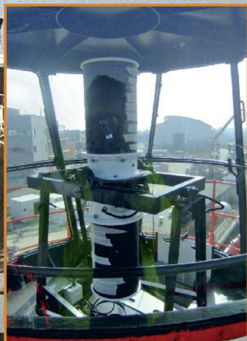
Above: Photographed during commissioning of the new gimbal mounted LED MSM light in a 20 Class lightvessel and showing overall configuration. The manufacturer was Mediterráneo Señales Marítimas of Spain.
