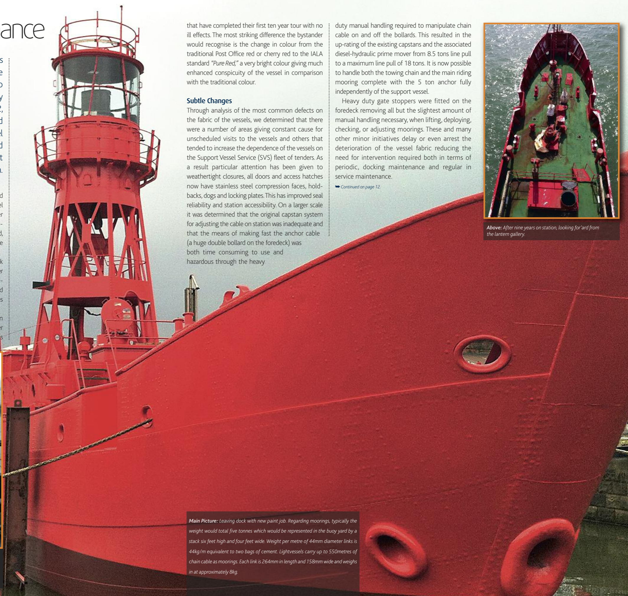
Above: In the lantern of a 20 Class lightvessel the LED MSM aid to navigation provides a 15mile light and comprises 11 rings of 10 LEDs each.
