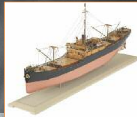
The D-type merchant vessel of 1917, model to a scale of 1:96. To ensure rapid replacement of the losses caused by German submarines in the First World War, a large number of merchantmen were built on a few standard designs. These workhorses of the world's oceans were given names ranging from War Acacia to War Zinnia (all active in 1917). The model represents the 'D'-type designed by S P Austin & Sons of Sunderland. It shows the defensive armament of a single 4.7 inch gun and the paravanes for protection against mines. It is of exceptional quality; the fittings, in particular, have been beautifully made. Illustrations © National Maritime Museum.
