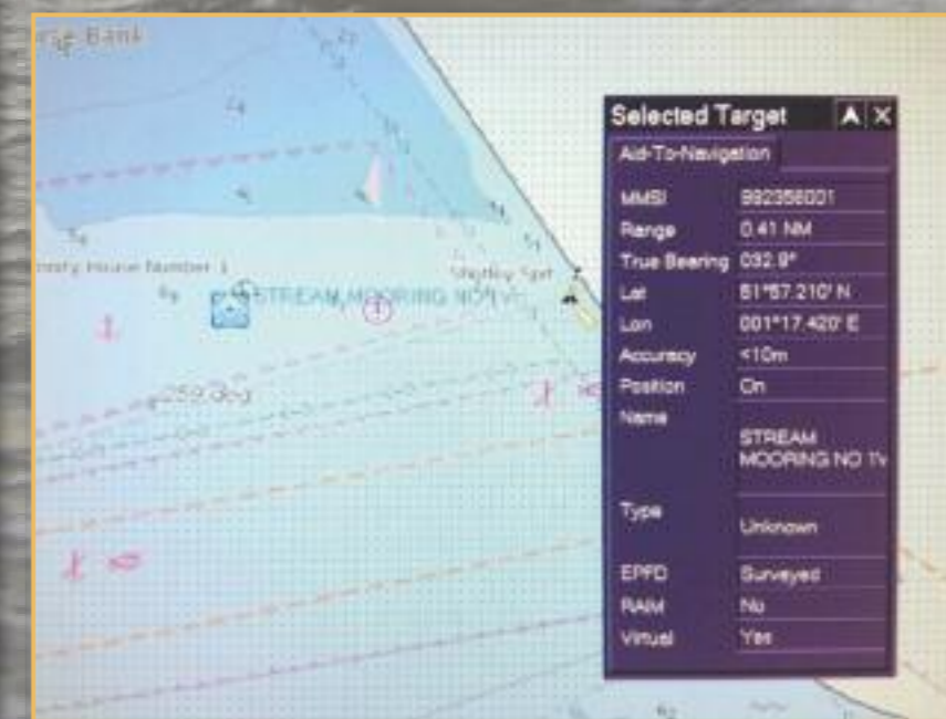
Figure 4: ECDIS showing Virtual AtoN transmitted by THV Alert on to Stream Mooring No. 1.
