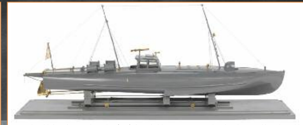
A superb model of a 55-foot coastal motor boat (CMB) of 1917, built by a variety of companies throughout the First World War. This model was made by John Thornycroft. In 1917 the 55-foot CMB was developed to give greater range and the model shows an early version of this type on its launching trolley. They had a crew of between three and five and some were capable of 40 knots. The boat is fitted with a trough housing an 18-inch torpedo. It had been necessary to develop an apparatus which, without the weight of a torpedo tube and without detracting from the boat's sea-going qualities, would launch a torpedo at speed. A twin Lewis gun-mounting sits on top of the cockpit. The need for this anti-aircraft defence had been demonstrated when a force of the earlier CMBs was annihilated by German seaplanes. The metal device on the front of the cockpit roof is a torpedo director, for calculating deflection to allow for the enemy's course and speed before firing. Four depth charges were carried and mines could be loaded instead of torpedoes. These CMBs gave useful service operating out of Dover and the East Coast ports, but their most successful exploits came later in the Baltic, against the Bolsheviks in 1919. A large force of 55-foot CMBs sank the battleships Petropavlovsk and Andrei Pervosvanni and a submarine depot ship in a single raid on Kronstadt Harbour.
