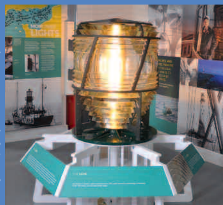
Lower left: Lens-based or 'dioptric' optics were invented in 1823; optics that were painstakingly constructed in the 19th century are still used widely today! This example is believed to have been installed at Monkstone beacon.
