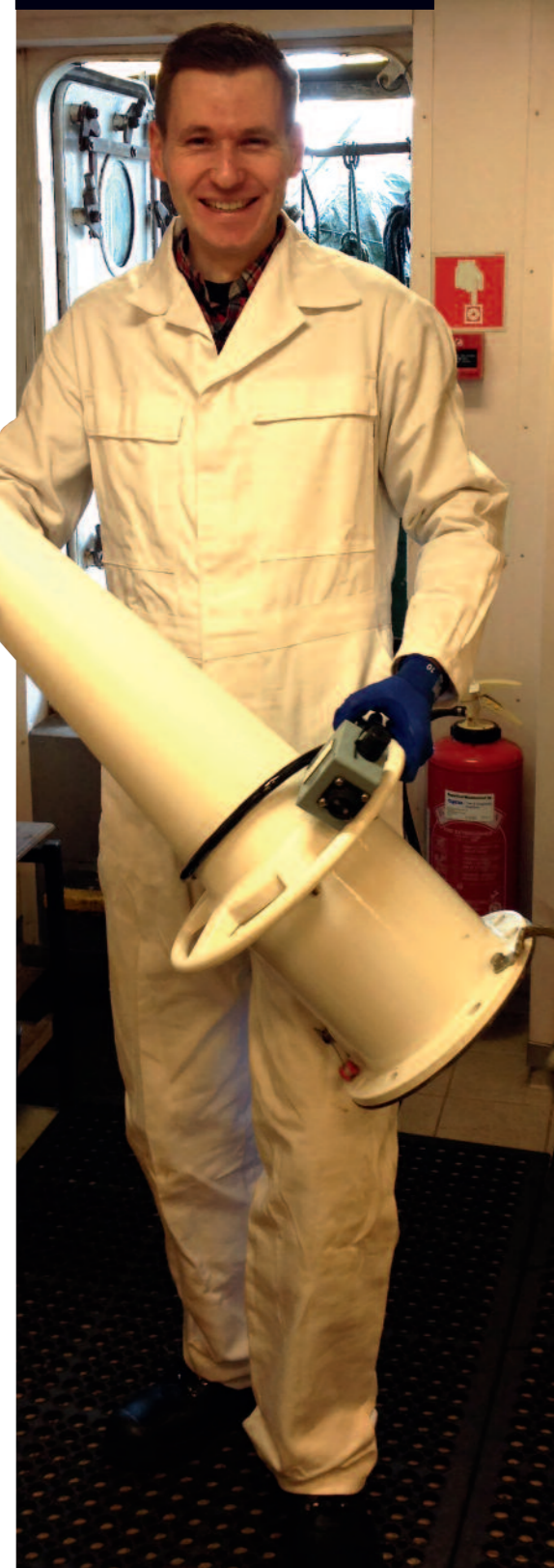
A Tideland Sea Beacon 2 System 6 radar beacon or racon being carried by Dr. Jan Šafář, R&RNAV Development Engineer. This unit has been modified to provide data on location, but that is not visible.
