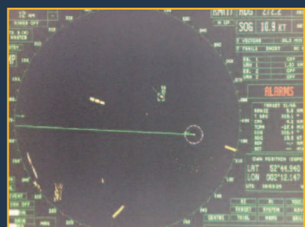
Above: The racon in question is between 9 and 10 o'clock (3 dashes). There are two other racons visible (long dashes) near the bottom and right-hand edge of the display. The green line is the Electronic Bearing line (EBL), which is set by the user. The vessel's position is the dashed circle at the origin of the EBL. The target above it is an AIS response from another vessel.
