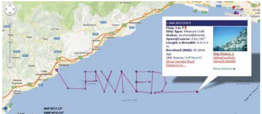
Figure 1: An example of hacking AIS, a false AIS signal is generated describing a vessel whose path spells out "pwned" (meaning "hacked"). ©M. Balduzzi et.al, "Hey Captain, Where's Your Ship? Attacking Vessel Tracking Systems for Fun and Profit," Hack In The Box , October 2013
