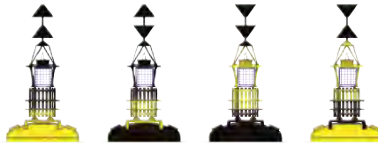
From left to right: North Cardinal, East Cardinal, South Cardinal, and West Cardinal Class Two buoys
