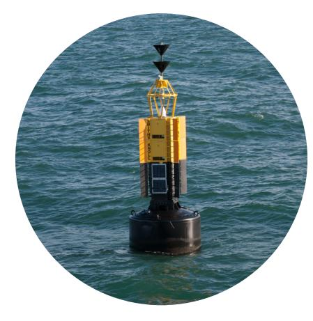
A buoy is a highly visual object that floats in water and is used to locate or warn passing ships. Buoys are generally bright in colour.
