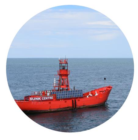
Trinity House has a number of lightvessels. These provide a visual aid to navigation in daylight hours in the form of a large red ship and by night they provide a long-range powerful light for ships in the area.
